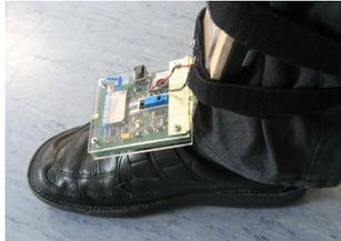
**Figure 8. Foot-attached RFID Reader**
