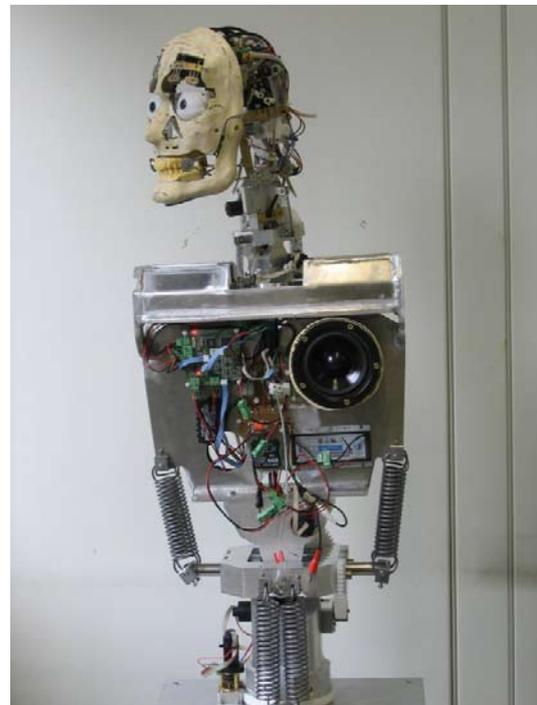
Figure 1: The skeleton of the humanoid robot ROMAN without clothes and silicon mask
