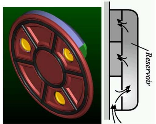
Figure 3: Mechanical design of the under pressure system. The 7 chambers are connected to a reservoir of 50l volume.
