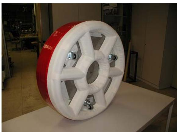
Figure 5: The testbed to examine the under pressure systems and the seals of the climbing robot.
