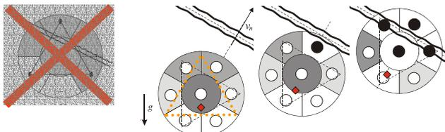
Figure 8: Optimal strategy of motion to overcome a crack. On the left figure only 2 chambers are generating the adhesion. After rotating the robot in the worst case 3 chambers are still generating the under pressure.
