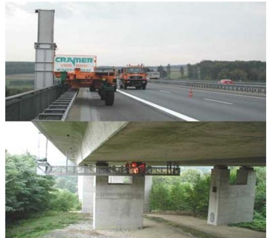
Figure 1: Device to access undersides of bridges.
