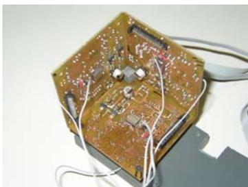
Figure 9: The inertial sensor system
