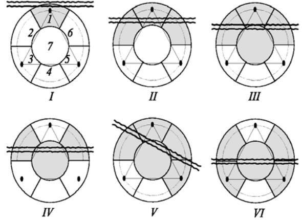
Figure 2: Simulation of the 7 chamber system climbing robot when moving on a vertical wall over a crack. The gray areas show those chambers which lost under pressure. It was calculated that in situation III, V and VI the robot is falling down.
