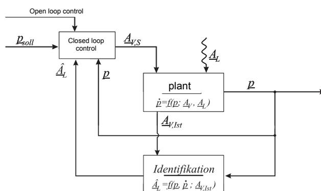
Figure 7: Closed loop control system for the under pressure system.
