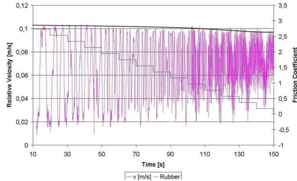
Fig. 5. Static friction: rubber to plane marble
