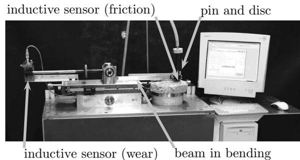
Fig. 2. Pin on Disc test stand
