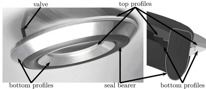
Fig. 1. Prototype and drawing of the basic construction
