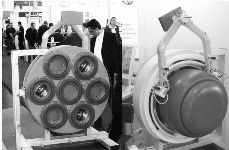
Fig. 10. CROMSCI platform as presented at the Hannover Messe 2007 with seven vacuum chambers, mounted sealings (left) and reservoir chamber (right).
