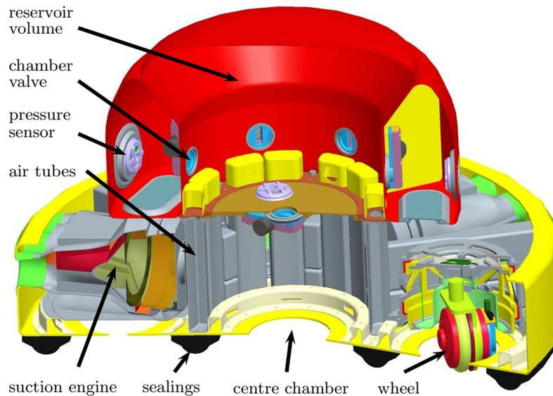
Fig. 2. CROMSCI's negative pressure system
