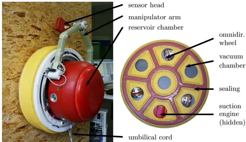
Fig. 1. CROMSCI sticking to a wall (left, view on top) and its sealing system (right, bottom view)
