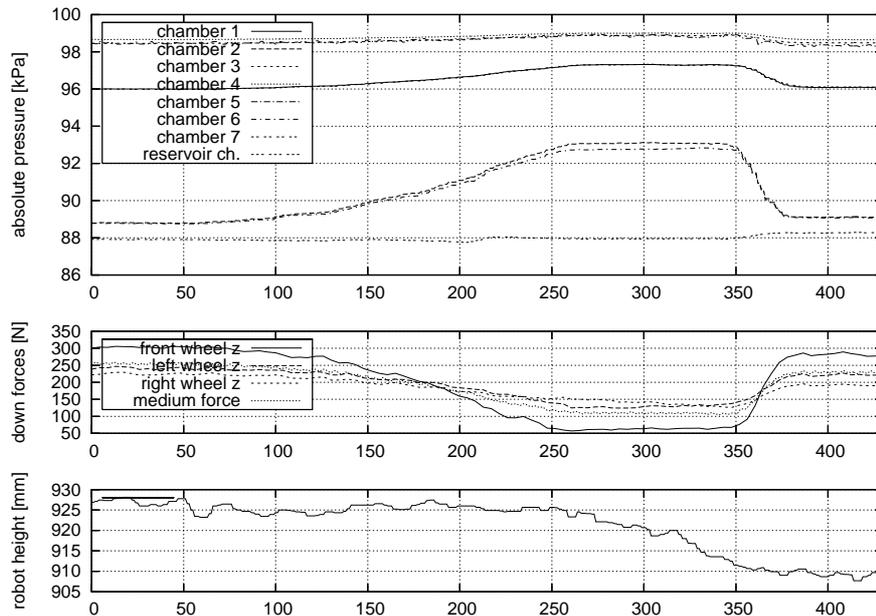
Fig. 4. Correlation of negative pressure, downforces and robot's behavior.
