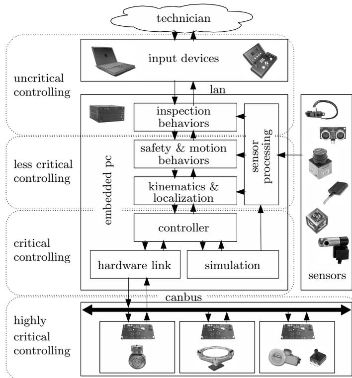
Fig. 3. Control structure of CROMSCI
