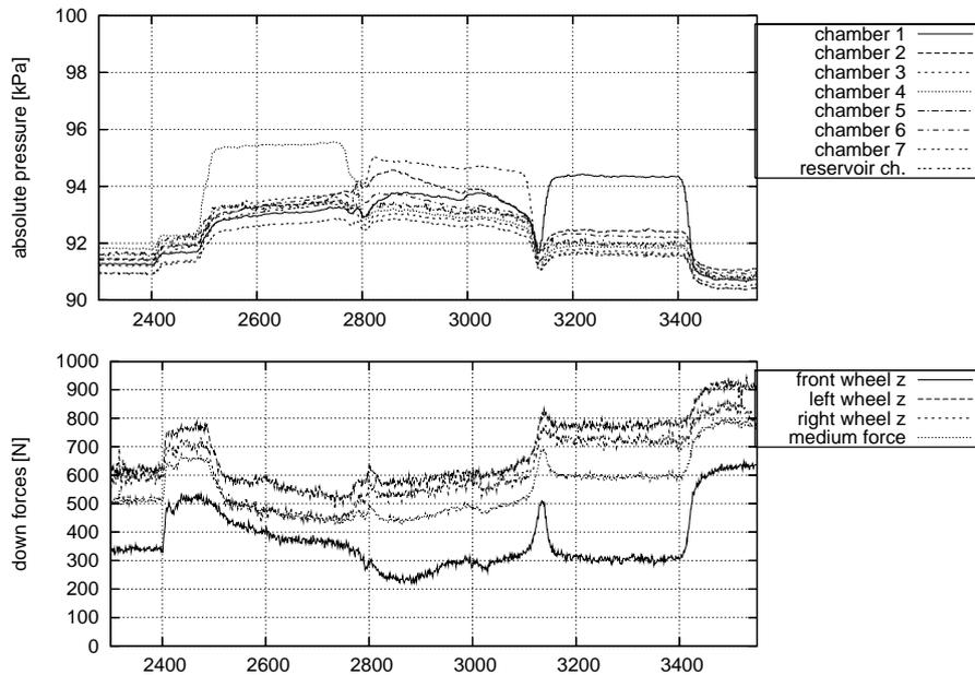
Fig. 5. Correlation of negative pressure and downforces while passing a leakage area.
