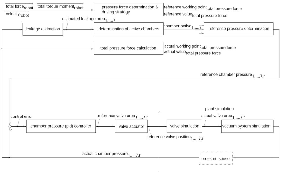
Figure 6: Structure of closed-loop pressure controller combined with simulation
