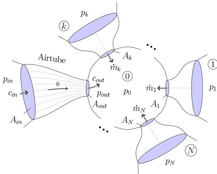
Figure 5: Modelling of airflow by an airtube
