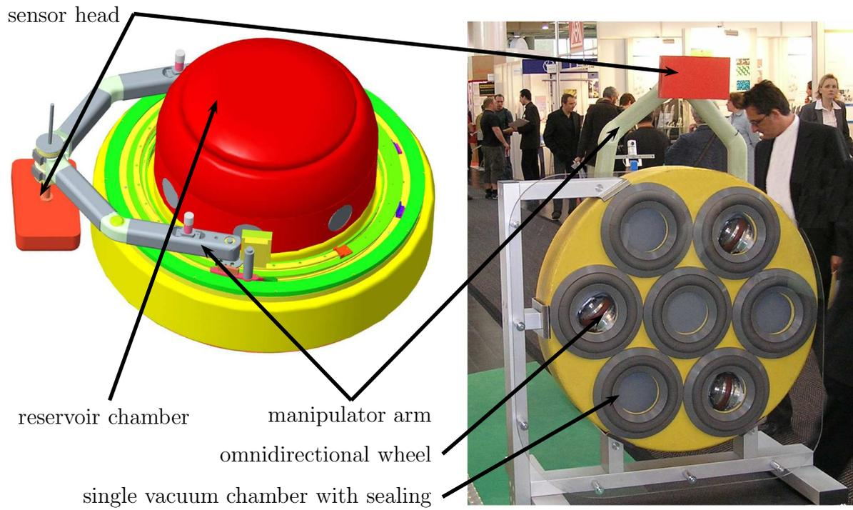
Figure 1: Construction drawing of CROMSCI (left, view on top) and as presented at the Hannover Messe 2007 (right, bottom view)
