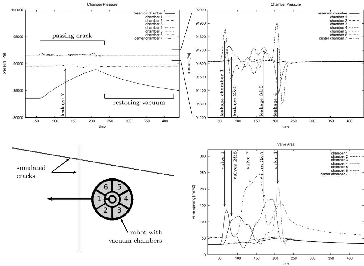
Figure 10: Simulated passing of a crack (bottom left) and resulting pressure values (top) and valve openings (bottom right)
