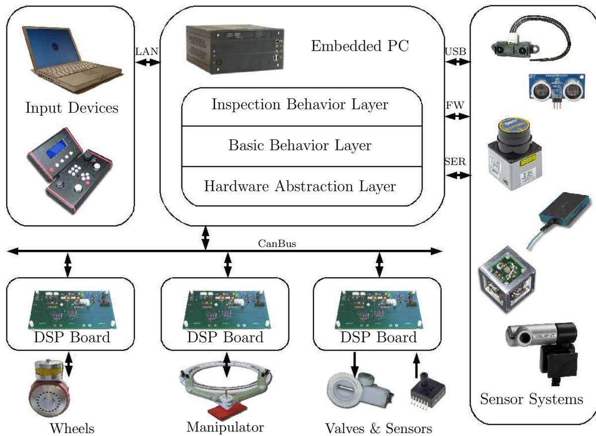
Figure 7: Overview of control architecture
