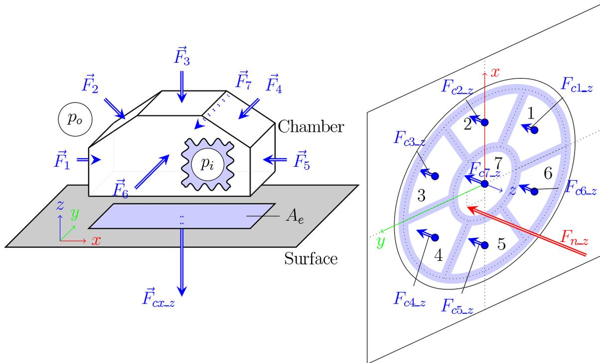
Figure 4: Forces which take effect on the robot
