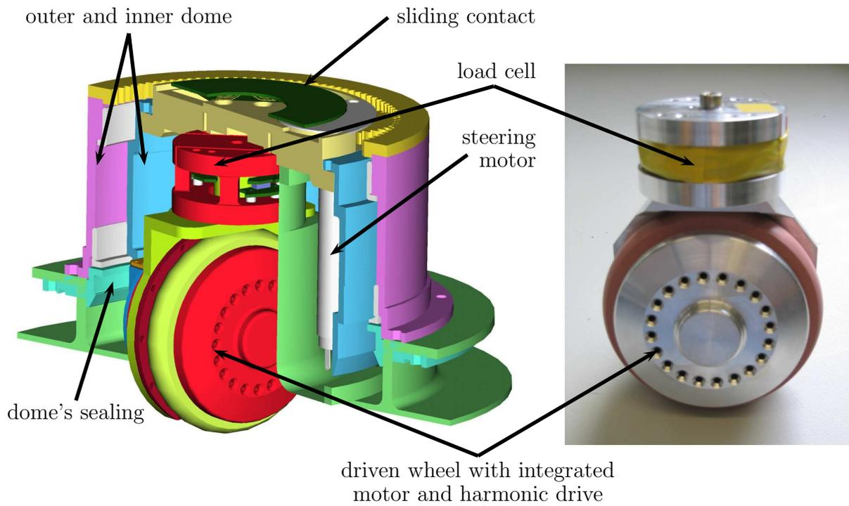
Figure 2: Construction drawing of a single wheel (left) and inner part (right)
