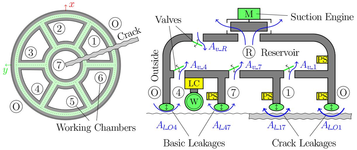
Figure 3: Division of suction chambers with an example crack (left) and overall elements and airflow (right)
