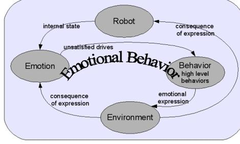
**Fig. 4.** The information flow for emotional behavior. An emotional behavior depends on the satisfaction of the different drives. If a drive is unsatisfied it tries to get satisfied again by changing the robots behavior.
