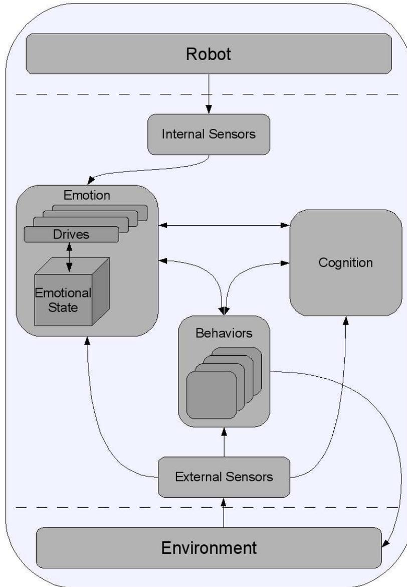
**Fig. 1.** The concept of the emotion based control architecture. The architecture consists of 3 main groups: Behavior, Emotion and Cognition. There are 3 layers of information flow within this groups: reflexes, emotional behavior and planned behavior.
