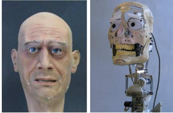
**Fig. 8.** The humanoid robot head "ROMAN" (ROMAN = ROBot huMan interAction machiNe) of the University of Kaiserslautern.
