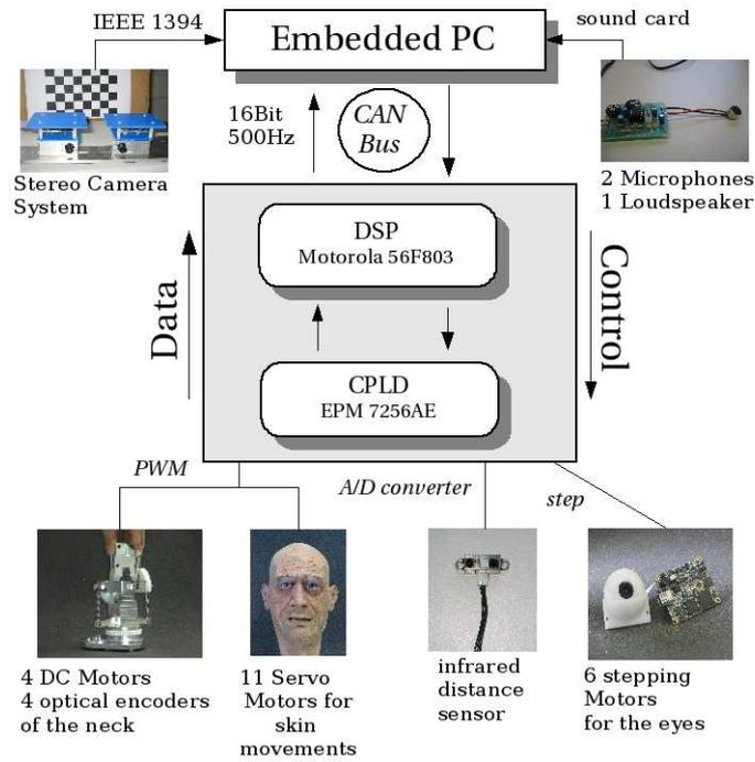
**Fig. 9.** Hardware architecture including sensor systems and actuators as well as all necessary connections to the embedded computer.
