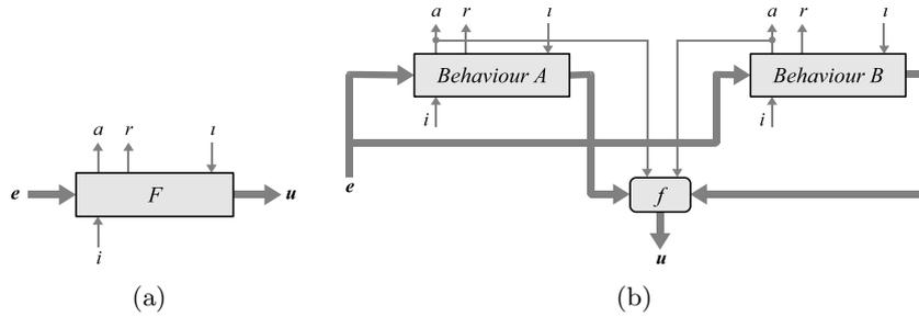
**Fig. 2.** 2(a): A single behavior node. All realized behaviors are build out of these modules. 2(b): The output of several modules can be merged by using a so called "Behavior Fusion"-Function  $f$ . The fusion depends on the activity of the modules. It could be either a winner takes all fusion or a weighted fusion.
