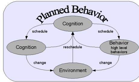
**Fig. 7.** The information flow for planned behavior. A planned behavior means that the robot changes behavior consciously to reach a certain goal.
