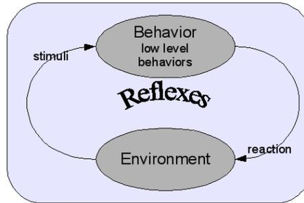
**Fig. 3.** The information flow of a reflex. A reflex is created just depending on sensor data.
