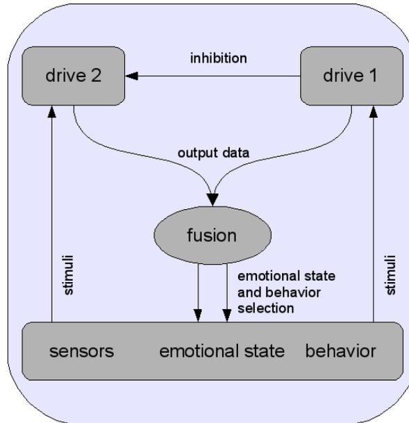
**Fig. 5.** The interaction of two drives, where "drive 1" has a higher priority level than "drive 2".
