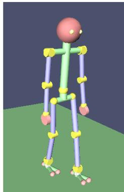
Fig. 2: The simulated biped featuring 21 degrees of freedom
