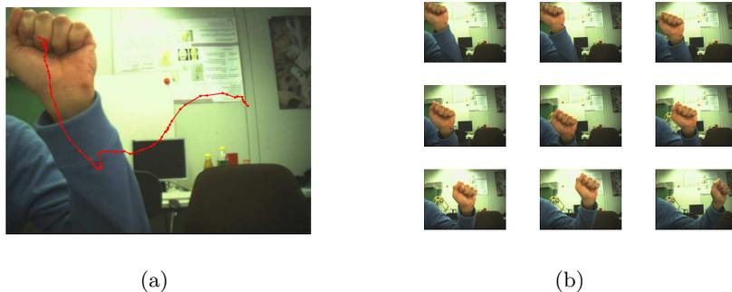
**Fig. 4.** (a) Input image captured from the camera. The motion of the hand is marked with a red line. (b) Images of the moving hand during the tracking process.
