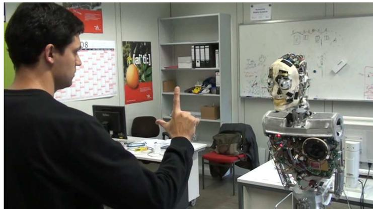
**Fig. 8.** Interaction between the robot and a human showing the L-gesture during an experiment.
