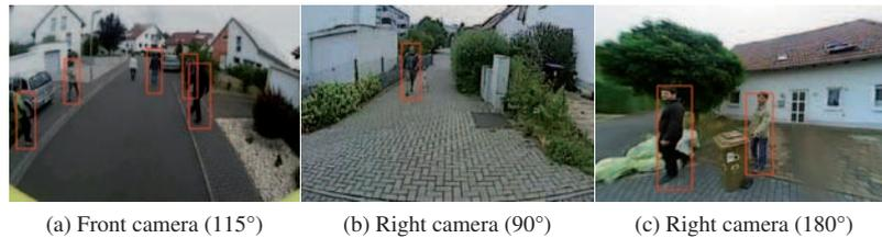
**Fig. 7.** Images of a refuse collection scenario using cameras with different opening angles and mounting positions. Red boxes mark pedestrians identified by the pedestrian detection algorithm.
