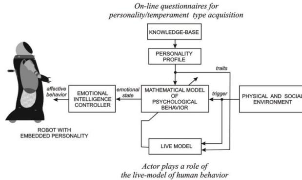
**Fig. 2.** Block-scheme of tuning the robot emotional intelligence controller based on personality traits acquired from biological model of human examinees.
