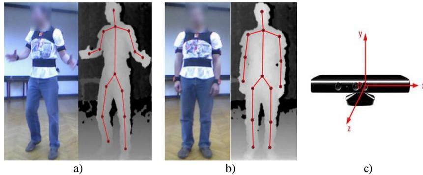
**Fig. 3.** (a-b) RGB streams (left) and depth streams with detected skeleton and collected joints (right) and c) Kinect device with axis orientations
