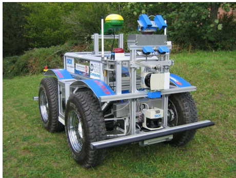
Figure 1. RAVON, the Robust Autonomous Vehicle for Off-road Navigation.
