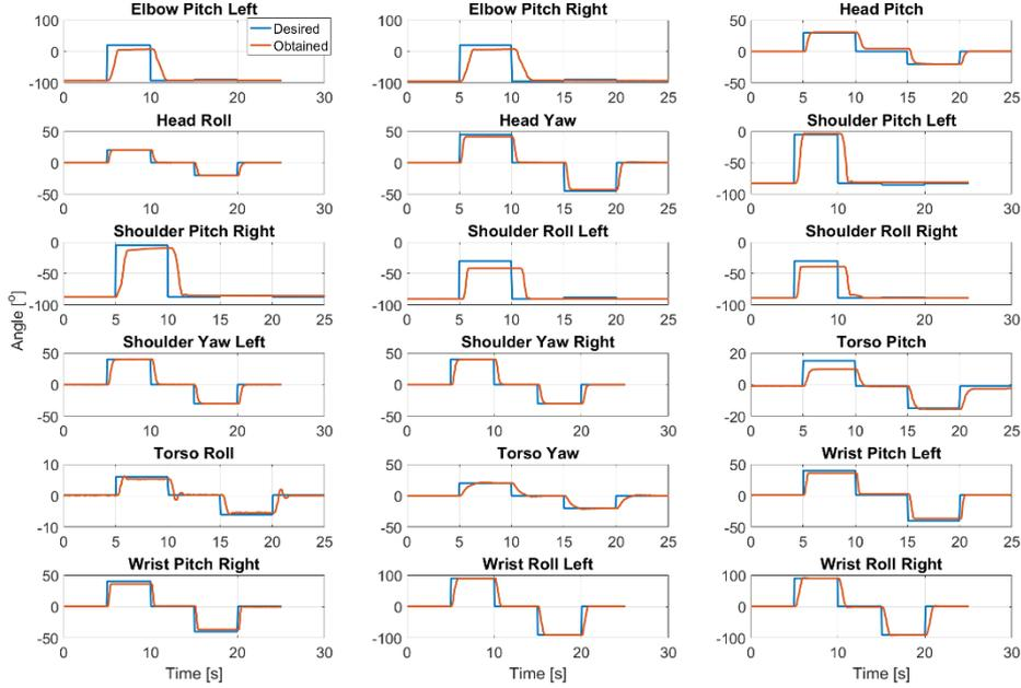
**Fig. 3.** Captured joint angle activation of RoboThespian
