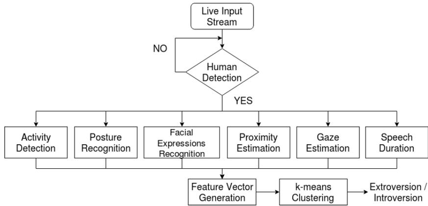
**Fig. 1.** Working schematics of proposed approach
