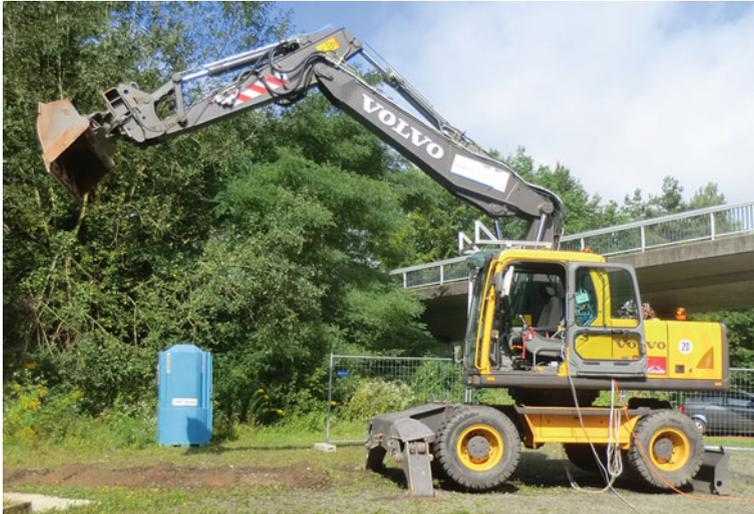
**Fig. 1** The autonomous bucket excavator THOR (*Terraforming Heavy Outdoor Robot*)
