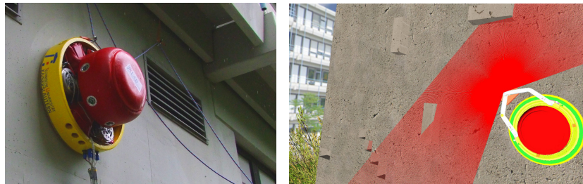
Fig. 1. Robot prototype CROMSCI driving at a concrete wall secured by a rope and supplied via umbilical cord (left) and 3d-simulation with visualization of scan lines (right)
