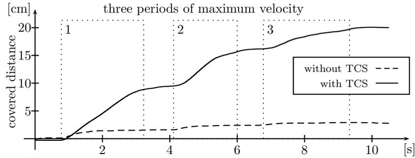
Fig. 5. The covered vertical distance with and without traction control system (TCS) performing stop-and-go at maximum velocity and acceleration three times
