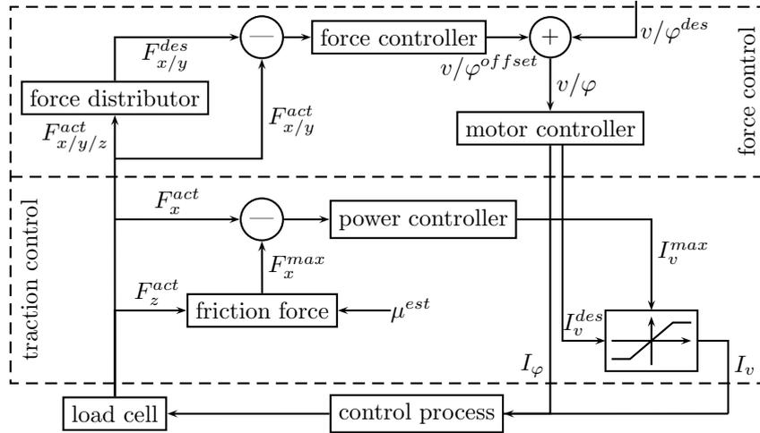
Fig. 4. Setup of combined shear force controller and traction control system (wheel indices are left out for clearness)
