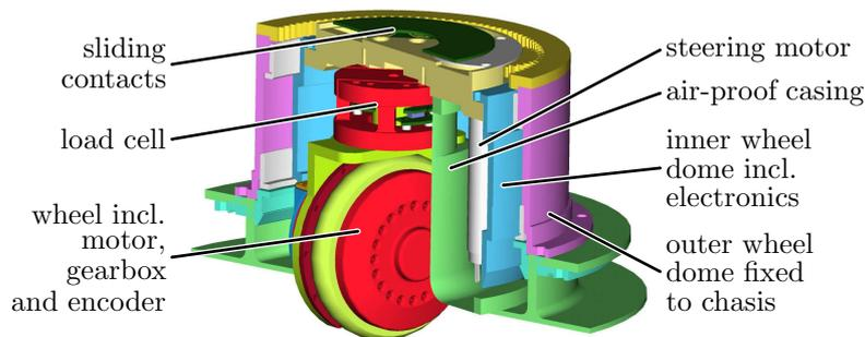
Fig. 2. The propulsion unit including wheel domes, load cell and inner wheel lying inside of an air-proof casing – the wheels are mounted inside of vacuum chambers
