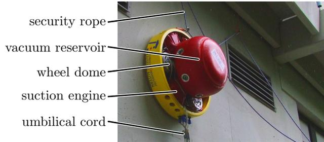
Fig. 1. Prototype CROMSCI (Climbing RObot with Multiple Sucking Chambers for Inspection tasks) driving at a concrete wall secured by a rope and supplied via umbilical cord (manipulator arm not mounted)
