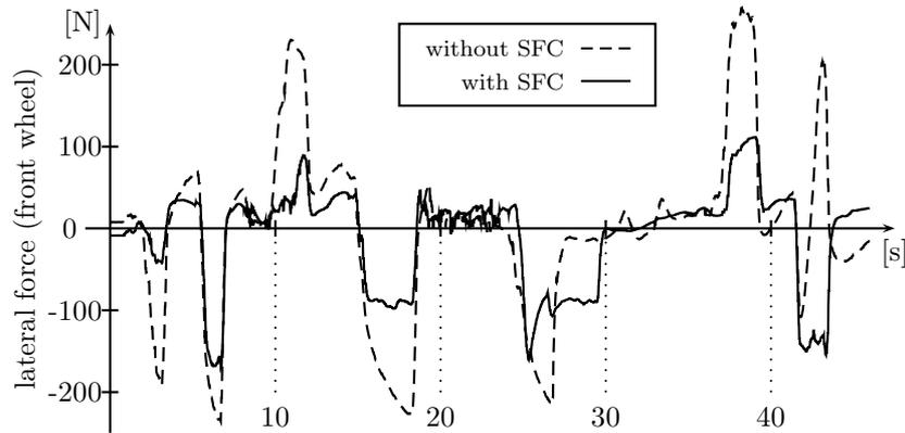
Fig. 6. The lateral forces of the front wheel while moving up a wall with permanently changing velocity and direction commands - with and without shear force control (SFC)
