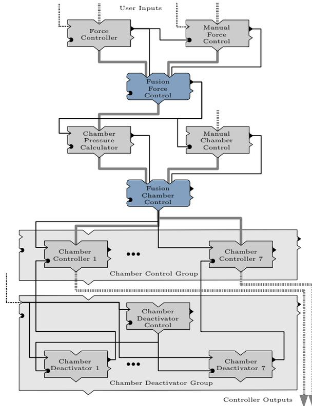
Fig. 3. Overall behavior structure of the negative pressure and force control system. The user can activate additional functionalities by stimulating the behaviors *force controller*, *manual force control* and the *chamber deactivator group*.
