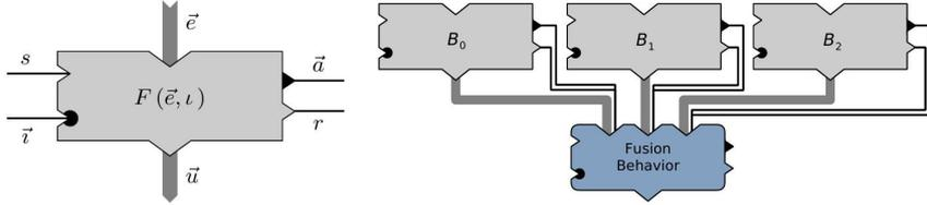
Fig. 2. Behavior module in the behavior-based architecture iB2C (left) and an exemplary fusion of the outputs of three behaviors by taking meta data into account (right)
