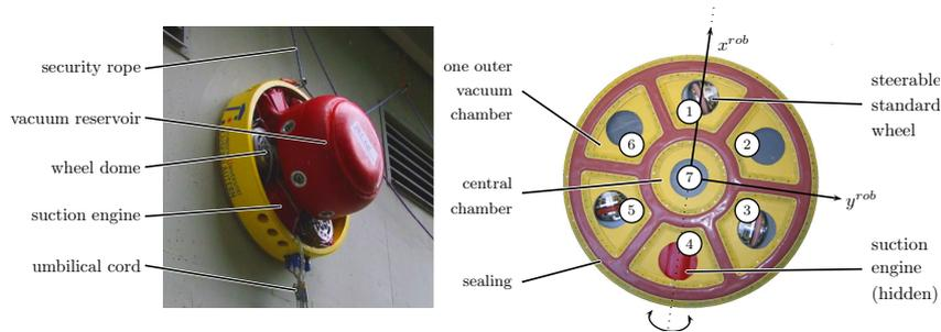
Fig. 1. Climbing robot CROMSCI in action (left) and the setup of the seven-chamber adhesion system (bottom view, right)
