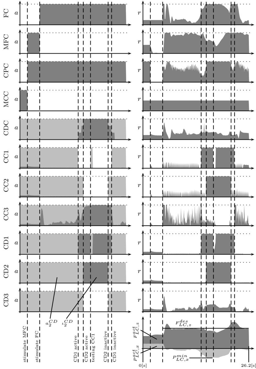
Fig. 4. Plot of behavior activities  $a$  (left, gray), activation (left, light gray) and target ratings  $r$  (right). On bottom right one can find the resulting downforce  $F_{LC,z}^{act}$  (dark gray graph) with a desired force of  $F_{LC,z}^{des} = 2200[N]$ . The light gray graph indicates the x-position of the downforce point which reaches a minimum of  $P_{LC,x}^{min} = -0.082[m]$ .
