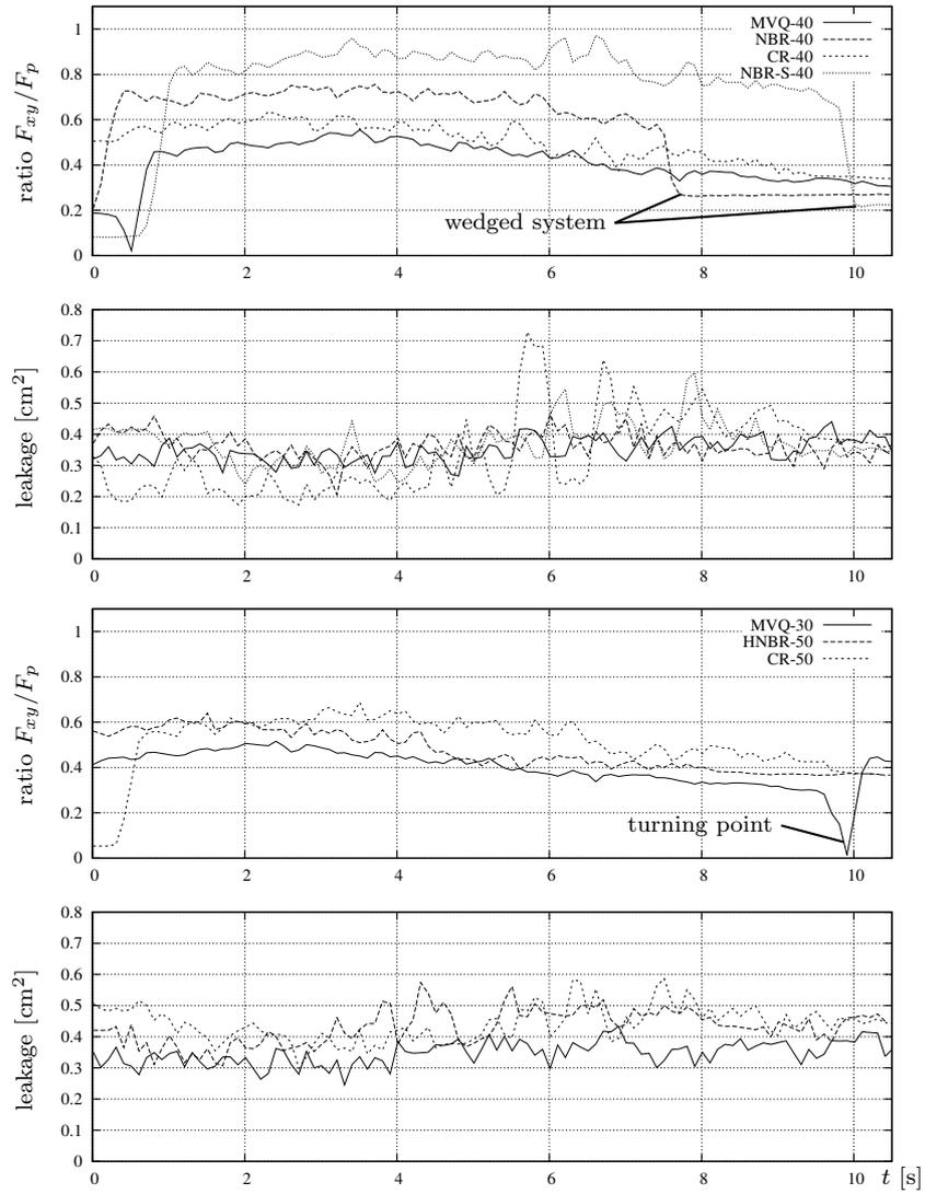
Fig. 5. Results of the dynamic experiments with adhered and moved platform using seven different materials.
