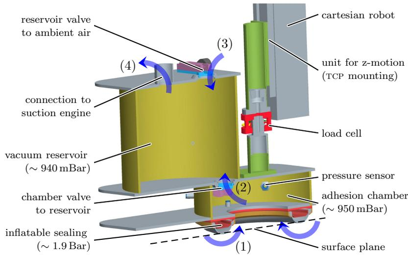
Fig. 3. Construction drawing of the adhesion system consisting of an adhesion chamber, a negative pressure reservoir and corresponding control elements.
