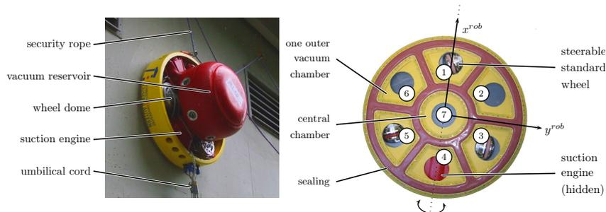
Fig. 1. CROMSCI (left) with its inflatable rubber sealing (bottom view, right)
