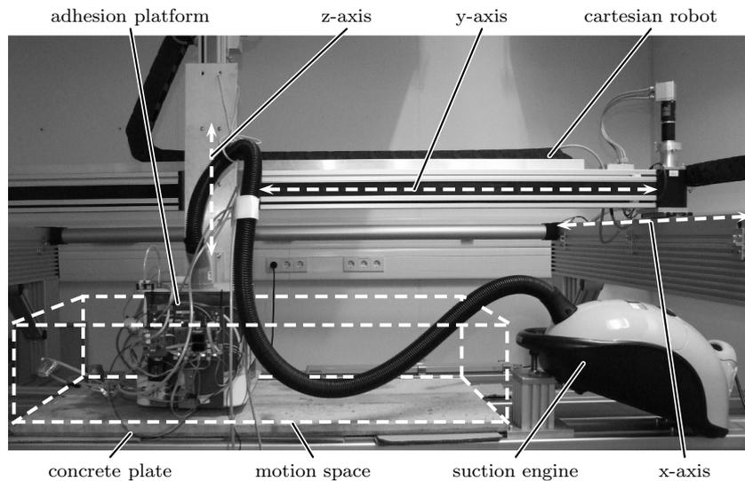
Fig. 2. The complete dynamic test stand with experimental platform (including the adhesion system), concrete surface, suction engine and cartesian robot with its three motion axes. The dashed box indicates the motion space of the platform.
