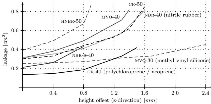
Fig. 4. Static leakages at varying distances between adhesion system and concrete plate with different sealing materials and shore hardnesses.
