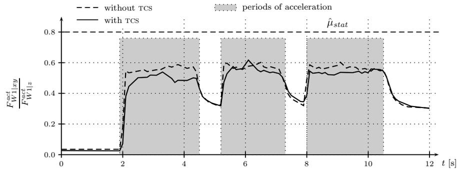
**Fig. 4.** Ratio of sideward forces to downforce of front wheel which has been enhanced from an average value of 0.56 during the three motion phases to 0.52 with activated traction control system.
