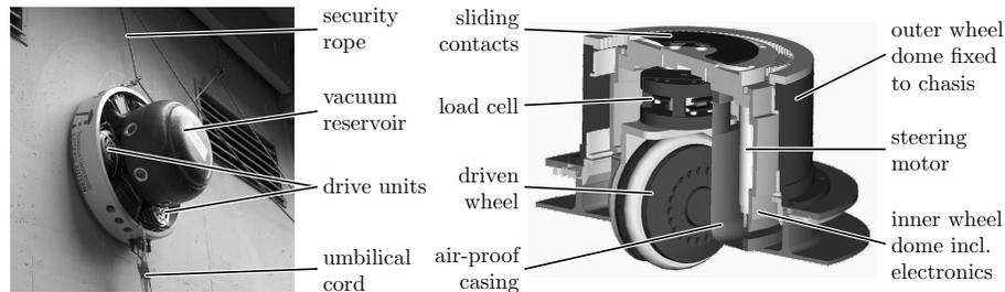
**Fig. 1.** Climbing robot CROMSCI at a concrete wall (left) and a drive unit for propulsion (right).
