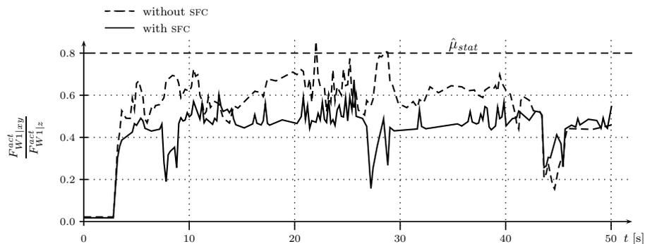
**Fig. 5.** Ratio of sideward forces to downforces while moving up a wall with permanently changing velocity and direction commands – with (solid line) and without (dashed line) shear force control. The SFC reduces this ratio significantly.
