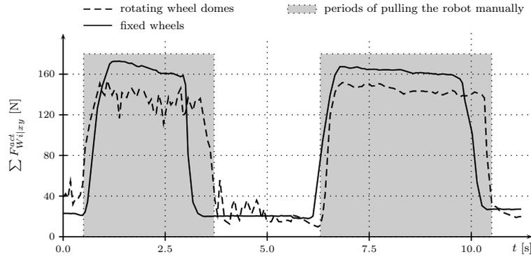
**Fig. 3.** Needed sideward forces to pull the robot by hand. In average the force is lowered from about 159.9 N (solid line) to 137.5 N if the wheel domes are turning (dashed line).
