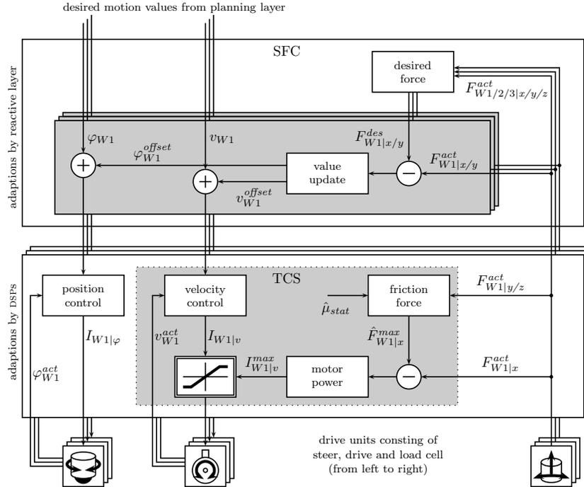
Fig. 2. Detailed view of the lower AMC elements traction and shear force control.
