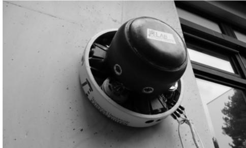
Figure 10: Real climbing robot CROMSCI navigating on a concrete wall.
